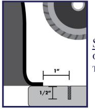
SLOT SPECIFICATIONS: USING AN APPROPRIATE BLADE, CUT A SLOT AT LEAST I/2" DEEP, I" FROM THE EDGE OF THE SINK RIM.
